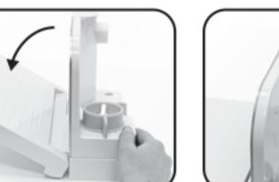
Align the blade with the blade-locking screw hole. Insert the blade-locking screw and turn clockwise untill it clicks to secure the blade on the unit.
