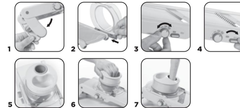
1. Unfold folding legs from underside of slicer.
