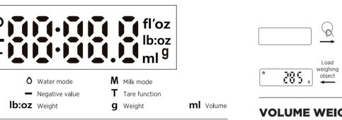
Press the circle button to turn on the scale.
